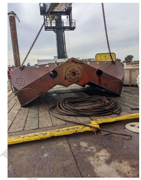
Figure 4- Closeup of an environmental clamshell dredging bucket. Photo by USACE Sacramento District.
