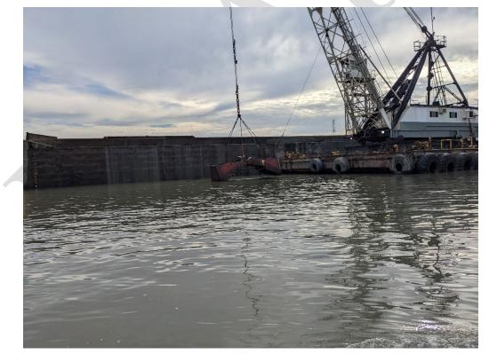
Figure 3- Mechanical clamshell dredger operating in a channel. Photo by USACE Sacramento District.
